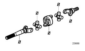
No service parts are offered for the new SX/DP-S/XDP u-joint.
