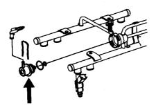
Testing has determined that the fuel screen on the Fuel Pressure Regulator can cause a restriction of the fuel return line. Restricting the return, line raises fuel pressure, which can degrade engine performance.
