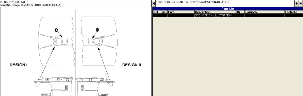
NOTE: TO INSURE ORDERING THE CORRECT REPLACEMENT GEAR HOUSING COMPONENTS, IDENTIFY YOUR GEAR HOUSING BY USING THE DIAGRAM ABOVE. IF YOUR GEAR HOUSING (DESIGN I - 3 JAW REVERSE CLUTCH) HAS A STRAIGHT MACHINED EDGE FOR TRIM TAB SCREW MOUNTING (A), ORDER FROM GEAR HOUSING BREAKDOWN PAGES (3 JAW REVERSE CLUTCH). IF YOUR GEAR HOUSING (DESIGN II - 6 JAW REVERSE CLUTCH) HAS AN ANGLED MACHINED EDGE (B) ORDER FROM GEAR HOUSING BREAKDOWN PAGES (6 JAW REVERSE
