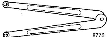
8775  | Removes and installs trim cylinder end caps.                                                                         |
