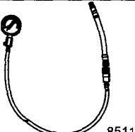
8511  | Checks cylinder compression. Use with M14 x 1.25 adapter.                                                                                  |
