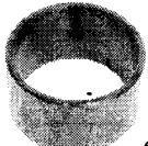
4739 | Compresses piston rings when installing the piston into the cylinder block.                                          |
