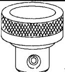
13667  | Aids in the installation of the propeller shaft needle bearing into the forward gear.         |
